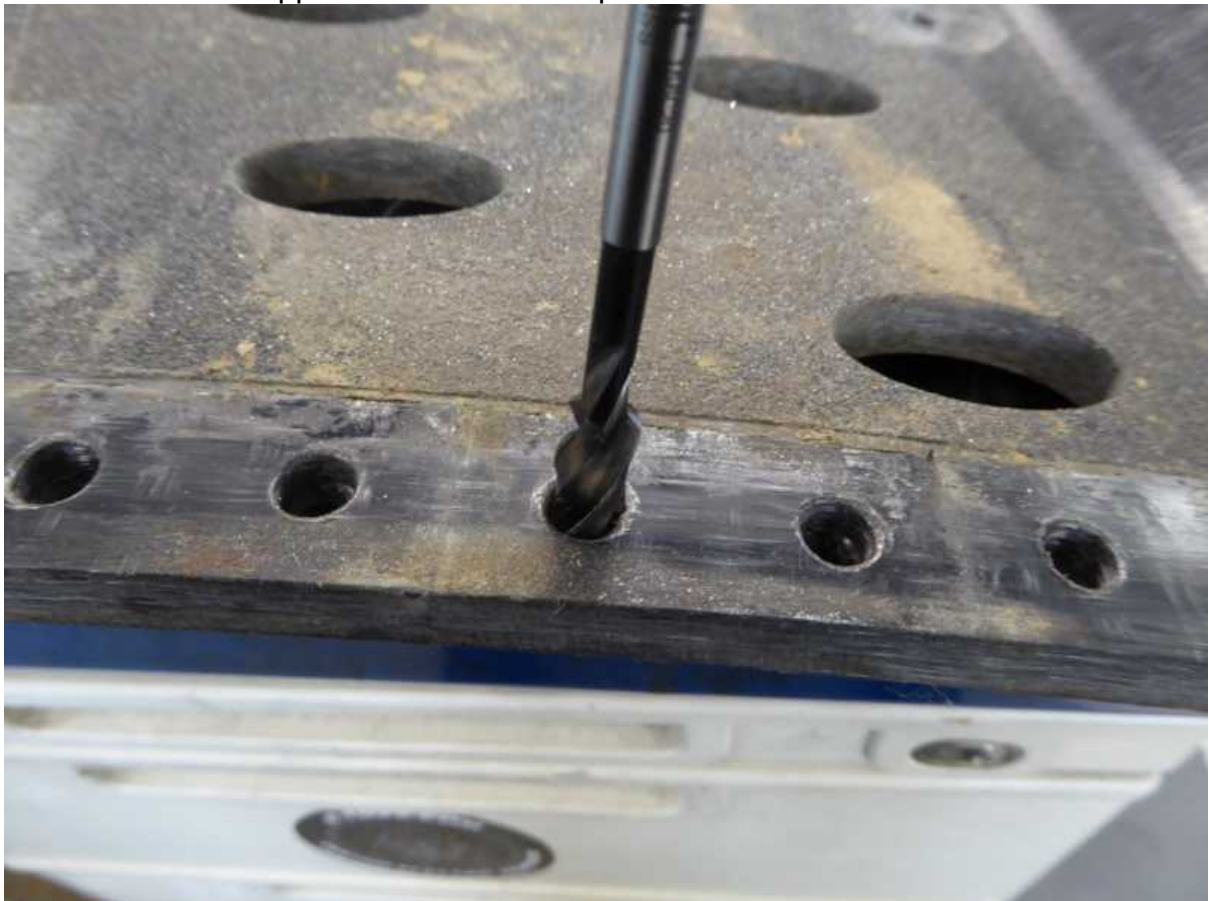
countersunk from upperside 5.5-6mm deep ...
