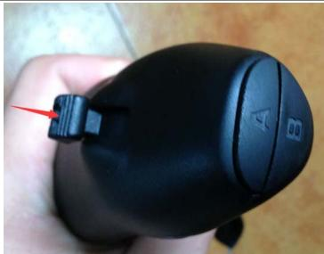
4. Press the B button 10 times in less than 10 seconds. All lights on your controller should turn off.
